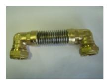
Connect the collectors hydraulically as per photo. Snug-tighten the screwed connection and then tighten it with a complete turn (mark nut and fitting).
